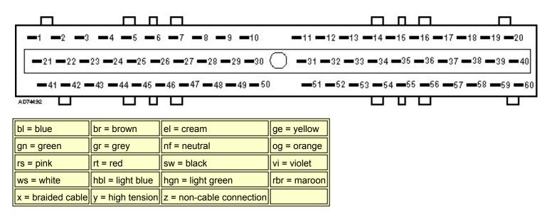
NOTE: In certain diagrams (Citroen, Peugeot & Renault), colour codes are replaced by numbers which are used to identify a particular cable and not the colour. In this instance, the cables will be numbered at each end close to the harness connector.
